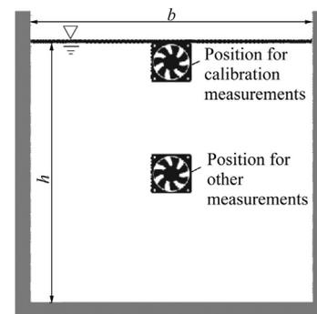
Fig. 2. Schematic diagram of experimental setup for velocity measurements (the grey areas indicate the walls of the tank).
