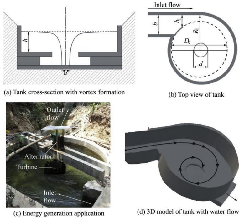
Fig. 1. Schematic diagrams defining geometrical variables of a circulation tank in which a vortex is formed, photograph of a system used for energy generation, and a 3D tank model with water flow indicated by arrows.
